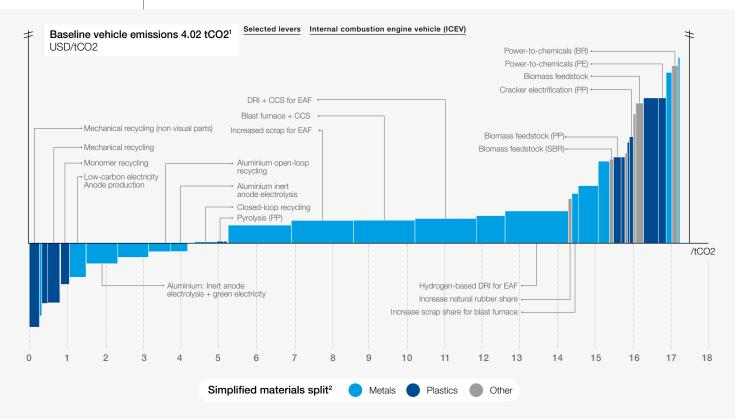
In this analysis, a premium C-segment vehicle with 1.95t vehicle weight: 1.04t steel; 0.29t aluminium; 0.10t rubber; 0.07t PP; 0.03t PE; 0.05t glass is considered
