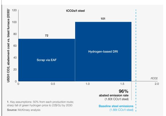
The levelized costs of hydrogen-based steelmaking would result in \$420–450/t steel, which may make this pathway more plausible than the (less technologically developed and economically feasible) CCS route. The primary obstacles for
