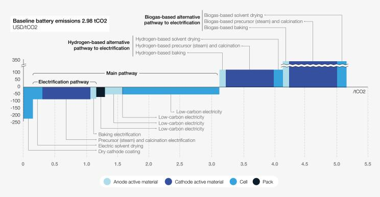
In this analysis a 92kWh battery per vehicle is considered, and only direct and indirect process emissions from fuels and electricity in the modelled production steps are included (mining or transport excluded)
