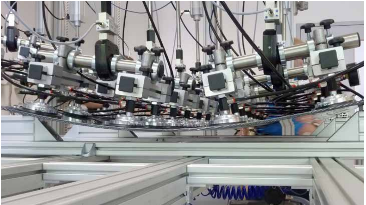
TPedge module passes a mechanical load test.
